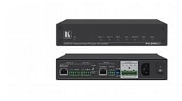
PA-240Net is a high-performance, selectable Hi-Z (70V/100V) or Lo-Z ( $4\Omega/8\Omega$ ) power amplifier featuring balanced and unbalanced inputs and additional line-level output and Dante interface. This versatile amplifier features built-in DSP, auto-standby and maximum durability. PA-240Net is suitable for a vast range of AV installations
